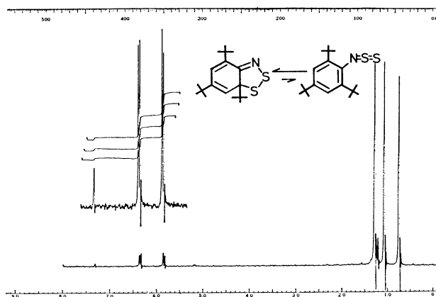
Fig. 1. NMR spectrum of an equilibrium mixture 1a + 1b in CD 2 Cl 2 (0.48 M) at 35 °C.
